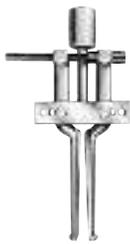
**Internal pulling attachments** have narrow jaws which extend through the center of the part to be pulled. They provide a straight pull and avoid damaging housings. Internal attachments feature adjustable jaws to fit various diameter parts. (page 200)
