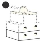
9510 and 9620 attach to the bottom of valve for remote mounting. The 9515 and 9521 mount between the pump cover plate and valve.
