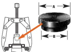
**Shaft protector set** -- Power Team shaft protectors are designed to protect shaft centers from distortion when extreme pressures are applied with jaw-type pullers or Push-Pullers®. Shaft protectors are inserted between the end of the puller screw and the shaft.
