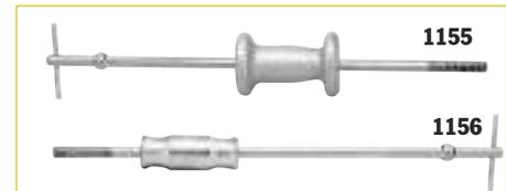
**Reversible-jaw slide hammer pullers** – Ideal for pulling gears, bearings, outer races, grease retainers, oil seals, etc. Two or three jaws may be used and positioned for “inside” or “outside” pulling jobs. Both have  $\frac{5}{8}$ "- 18 threaded end so attachments and adapters may be used.
