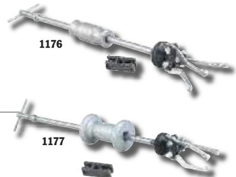
**Slide hammer pullers with cup pulling attachments** – These combine a basic slide hammer with No. 1152 internal pulling attachment for removing oil seals, outer races, and bearing cups from blind holes.
