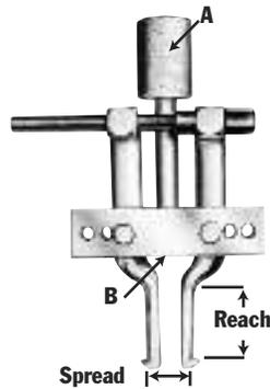
**CAUTION** – These attachments may not withstand the full tonnage of the pullers they are used with. The shape and condition of the part being pulled affects the tonnage at which the jaws may slip off. Always select the largest attachment which will fit behind the part being pulled.
