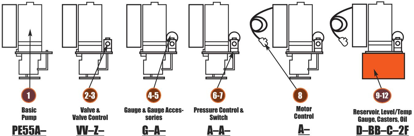
**Pump No. PE55A-VV-Z-G-A-A-A-D-BB-C-2F** is a 10,000 psi two-speed pump with a 115 volt, 50-60Hz, single phase, 1½ hp, 12,000 rpm motor; a 9512 4-way solenoid valve with a 202778 remote hand control, a 9041 pressure
