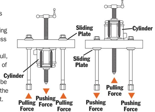
**Selection and capacity rating** – Each Push-Puller's specified tonnage "capacity" is determined using its standard legs in tension. Using longer legs, or a setup in which the legs are in compression, will reduce the "capacity". Always select the largest "capacity" puller and the shortest legs that will fit the job.
