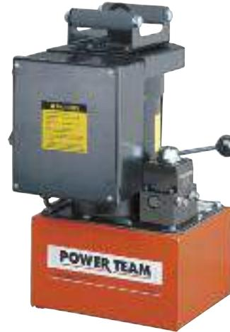
**PE60 Series** – The Vanguard® Supreme® pumps provide trouble-free service in the most severe working environments. Powered by a 1<sup>1</sup>/<sub>8</sub> hp, single phase motor, has a moderate noise level of 80-85 dBA. Start well under load even at the reduced voltages encountered on construction sites. High-output pumps, ideal for use with post-tensioning/pre-stressing jacks and other high-pressure hydraulic tools. See pages 84-85.
