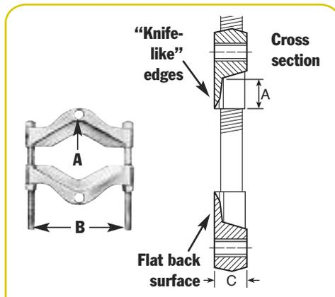
**Attachment clamps down into V-groove to distribute load. Use with Grip-O-Matic® pullers or Push-Pullers.**
