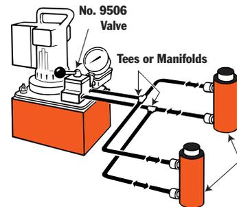
**3** Single-acting cylinder controlled by a remote mounted valve.
