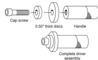
These sets have the proper-size driver for any seal, bearing or bushing installing job. Select the proper-size discs, attach to handle with cap screws and strike with hammer.
