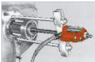
Typical setup for removing sprocket drive pinion shaft. Puller screw is attached to shaft by threaded adapter. Shaft is now ready to be pulled out hydraulically.
